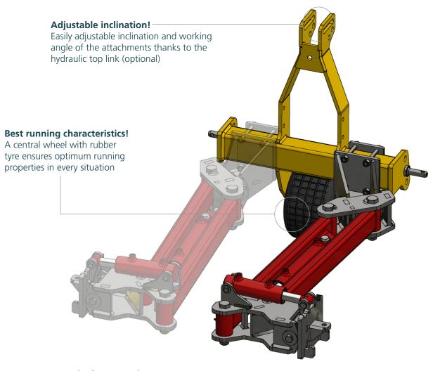
**Single suspension!** Freely movable carrier arms for perfect adjustment of the attachments to the ground contours, even in the most difficult conditions
