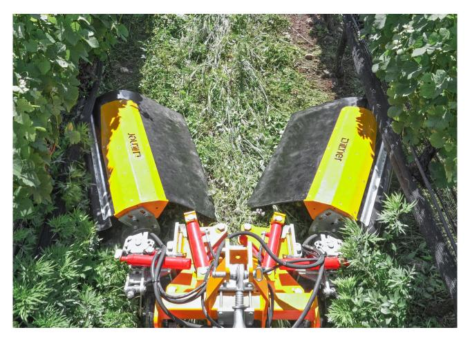
**Extremely compact!** For maximum maneuvrability and optimum undervine-care, from a row width of 1,50 m.
